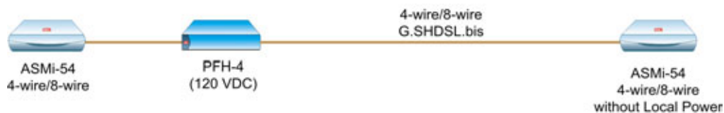
Figure 2. Remote Power Feeding for 4-wire/8-wire SHDSL.bis Lines
