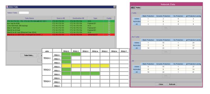
Figure 2. SDH Tunneling and Network Service View
